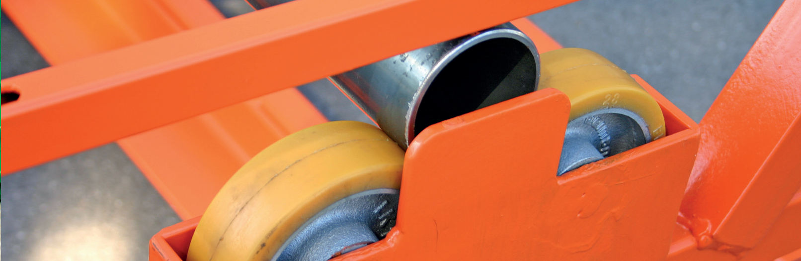
Braked or unbraked unwinding device, adapted to suit customer requirements
