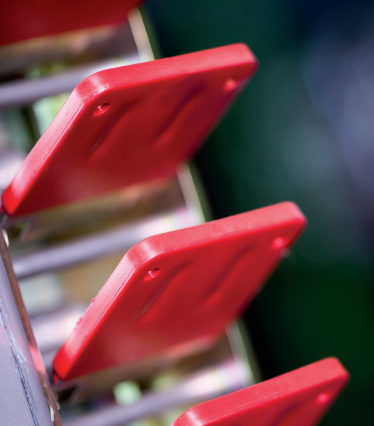
Transport rack for vehicle roofs with handle columns for robot loading and unloading
